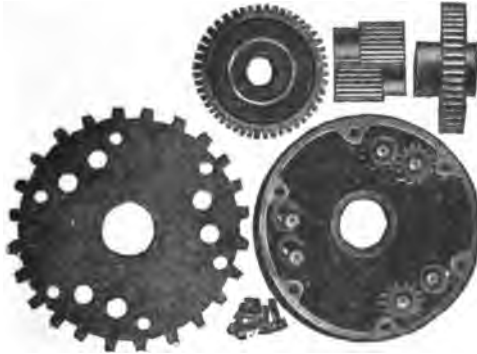
FIG. 26.—One form of Spur Differential or Balance Gear. The two inner ends of the divided axle shaft carry spur wheels, which mesh each with one of every pair of the three pairs of open pinions shown. As these pinions mesh together both rotate on their axes as soon as turning of the wagon begins.
